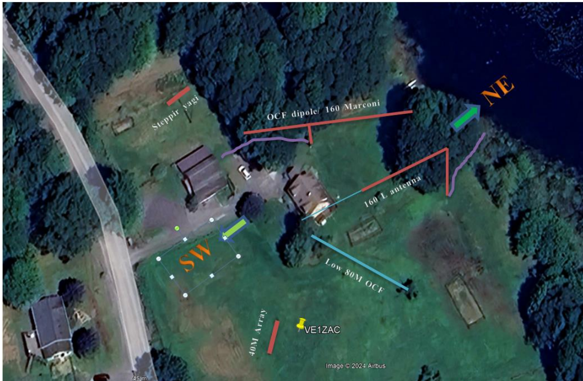
Figure 7 Oblique layout view. Purple lines are radials
