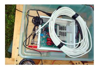
The inside of the base container showing the stub, the choke and the MFJ927 that destroyed itself last year. It's now replaced by an SGC239 Smart tuner, with the addition of a bias T and some RF connectors. (Note, there is a detailed explanation of this antenna, plus problems encountered with the first MFJ auto tuner on my VE1ZAC website)
